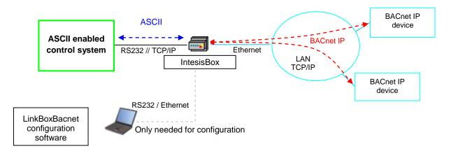
Points in BACnet can be read/written from an ASCII enabled control system using simple text messages. IntesisBox is a BACnet IP client device allowing read/write points of other BACnet IP device(s) connected to a BACnet network, and offering these point's values through its ASCII interface. ASCII interface of IntesisBox uses serial RS232 (baud rate configurable) or TCP/IP communication. For this application Daikin VRV system must be equipped with Daikin BACnet gateway DMS502B51.
